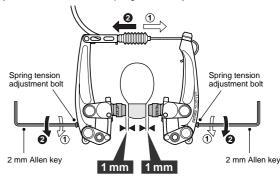
Depress the brake lever about 10 times as far as the grip and check that everything is operating correctly and that the shoe clearance is correct before using the brakes.
