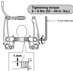
4. Pass the inner cable through the inner cable lead, and after setting so that the total of the clearances between the left and right shoes and the rim is 2 mm, tighten the cable fixing bolt.
