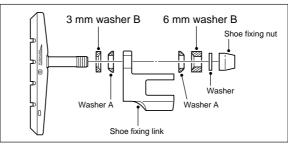
3. While holding the shoe against the rim, tighten the shoe fixing nut.
