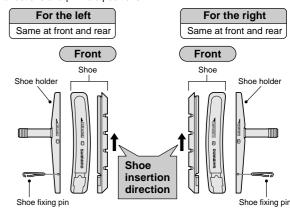
4. Insertion of shoe fixing pin is very critical to keep shoe properly fixed in place.
