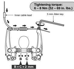
5. Adjust the balance with the spring tension adjustment bolts.
