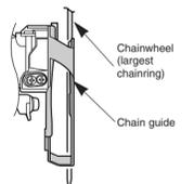
Adjust and then install the front derailleur as shown in the illustration. Do not remove the Pro-Set alignment block at this time.
