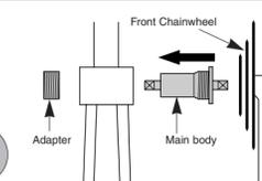
Use an 8 mm Allen key to install the front chainwheel.
