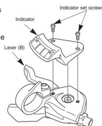
4. After checking that the indicator needle is at the right edge, install the indicator as shown in the illustration.
