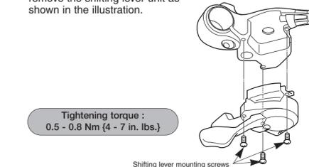
Tightening torque :
