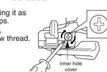
**Inserting the inner cable**
